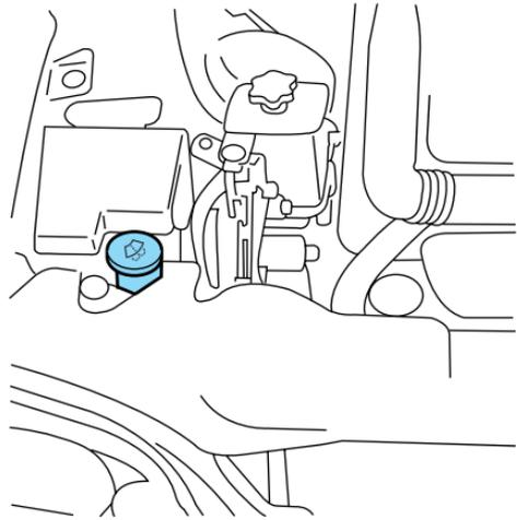
Only use a washer fluid that meets Ford specification ESR-M17P5-A. Refer to *Lubricant specifications* in this chapter.
