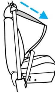
In this mode, the shoulder belt is automatically pre-locked. The belt will still retract to remove any slack in the shoulder belt.
