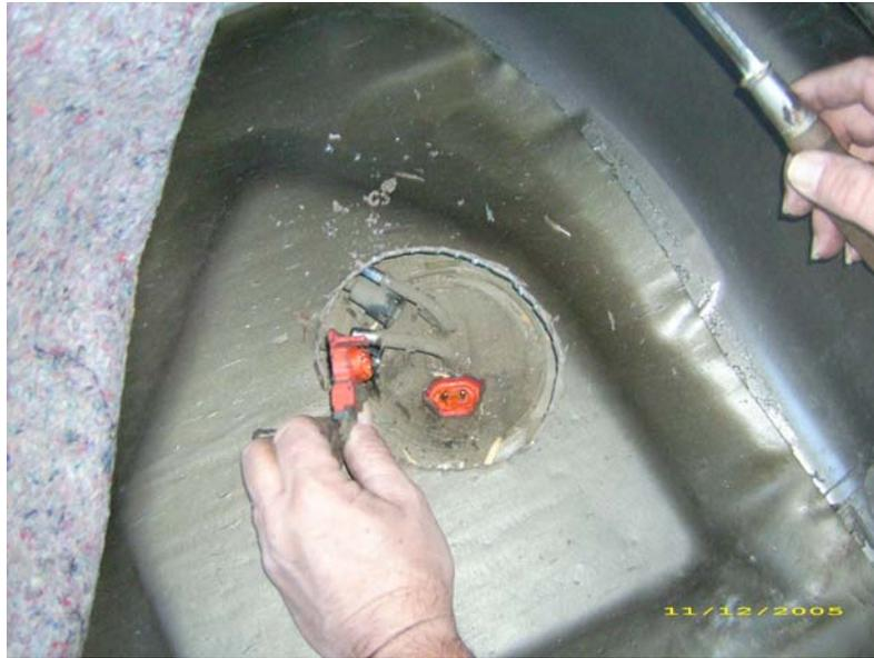
Using a drift or a screwdriver and a hammer, tap the retaining ring counter clockwise until it is free. Gently dislodge the pump assembly. The retaining ring is shown (below) hanging free on the pump assembly.
