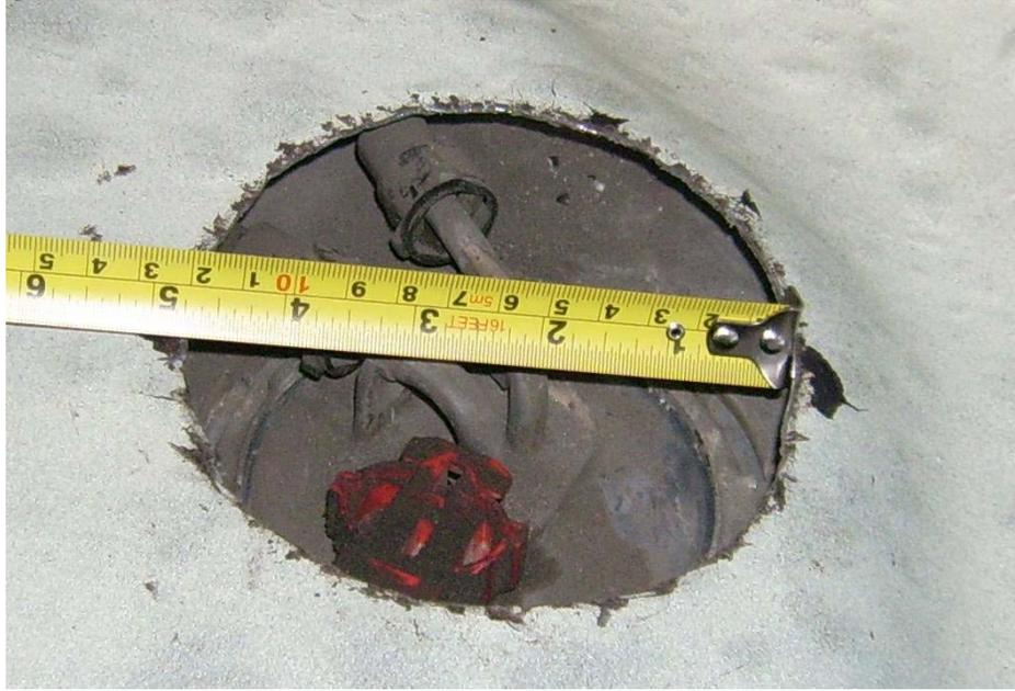
The clearance between the fuel connectors and the trunk floor is less than one-quarter inch. (1/4")
