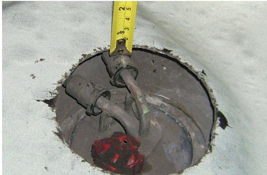
If you are removing the pump at this time, clean the area, remove the clips which secure the fuel connectors, and carefully slide the fuel connectors off with a twisting motion.
