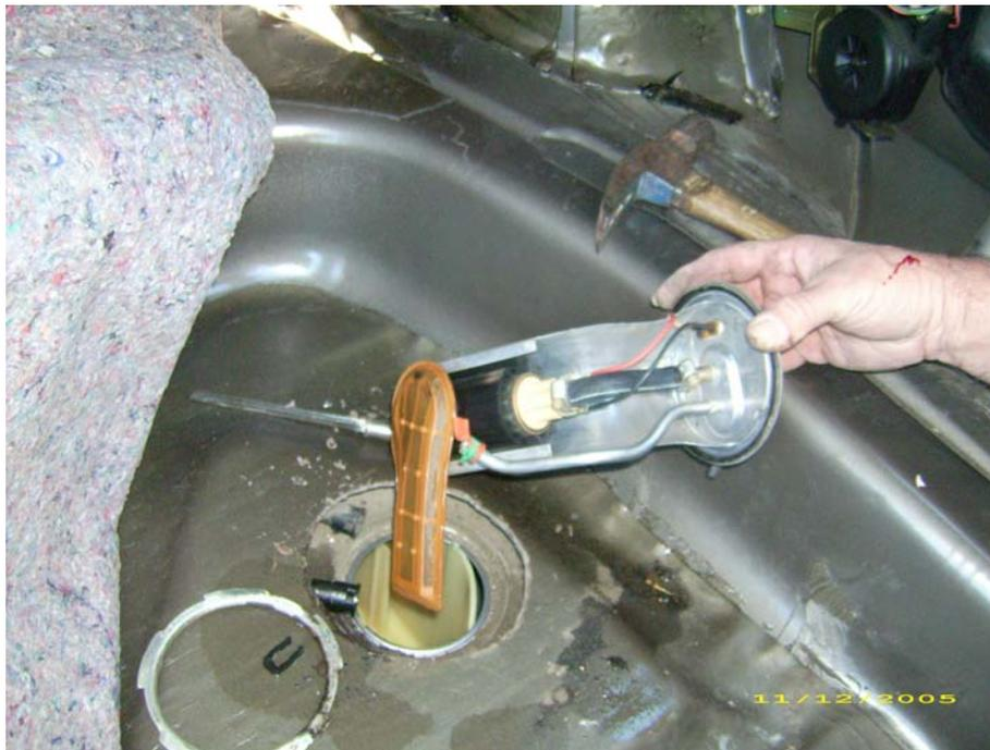
Install the replacement fuel pump per manufacturers instructions and re-install pump assembly using a NEW “square cut” O-ring.
