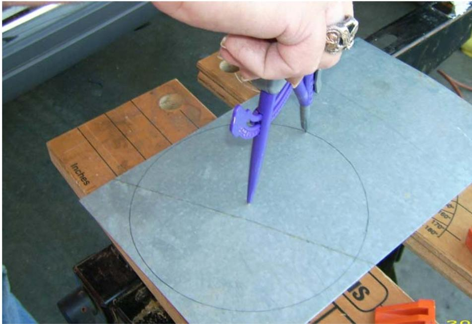
Using snips or any other method, cut the sheet metal into a disk.
