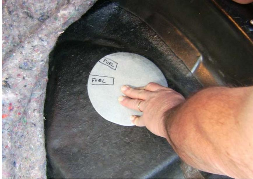
Punch or drill clearance holes for #6 sheet metal screws around the parameter of the cover, avoiding the fuel markings.
