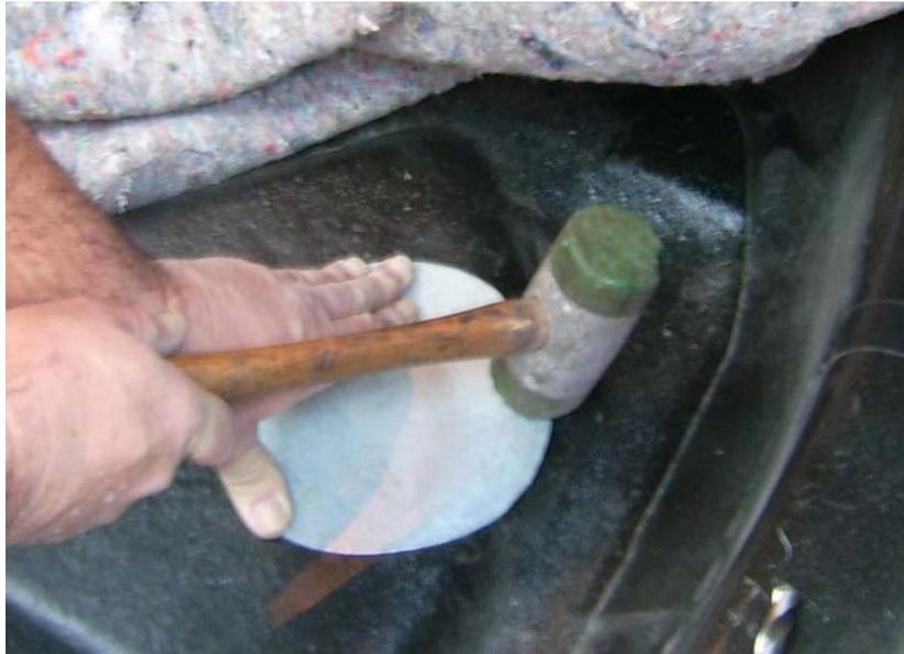
Placing the contoured cover in place. Mark the location of the fuel connectors on the cover as to make sure that you do not drill screw holes where the screws might puncture the fuel connectors or tubes.
