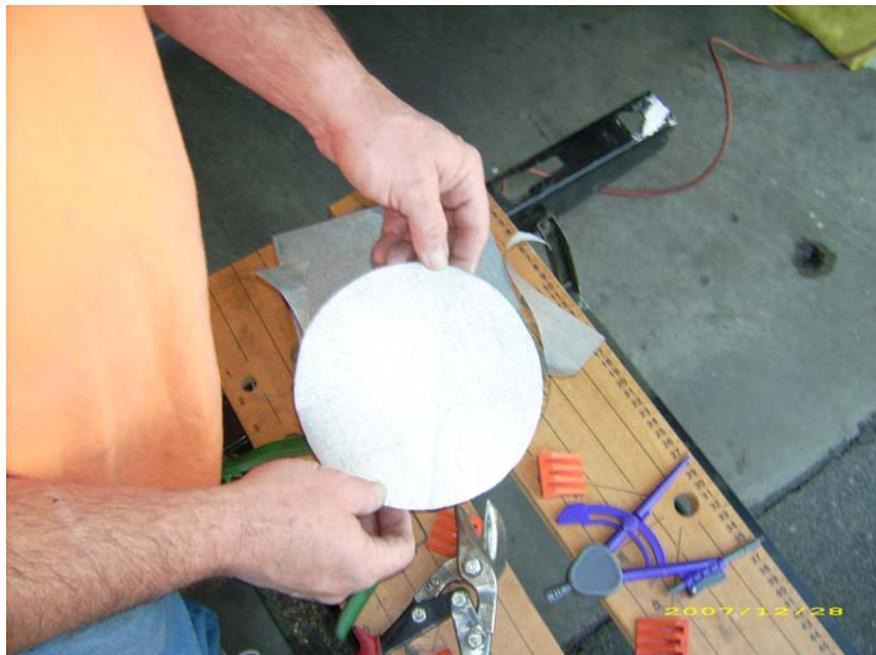
Locate the disk over the access hole. Using pliers, hammers or whatever means available to you, form the cover to fit the contour of the trunk. I used pliers and a soft faced hammer.
