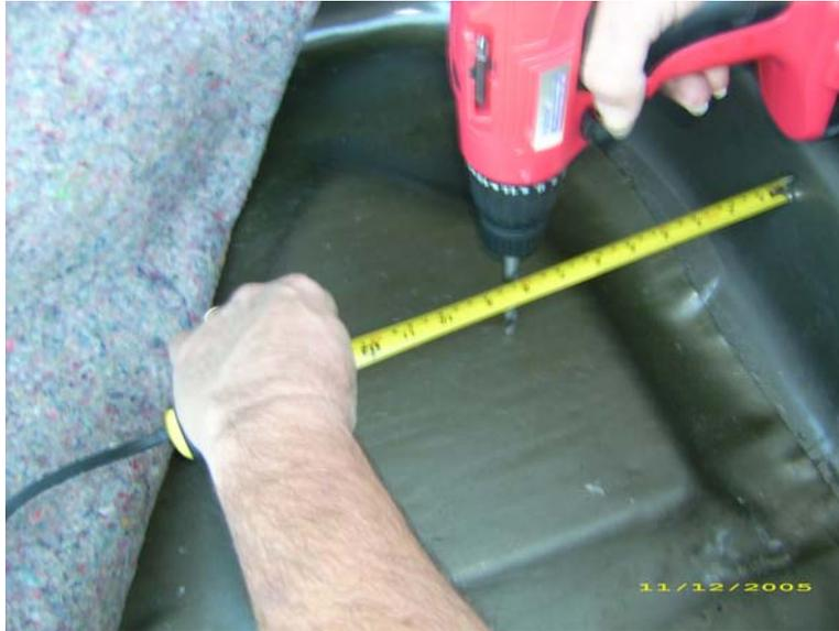
Measure 13-1/2" in from the forward side of the trunk well and carefully drill a 3/8" or larger hole at the 8" mark. Make sure not to let the drill bit grab and "pull" itself through the sheet metal, damaging the tank below.
