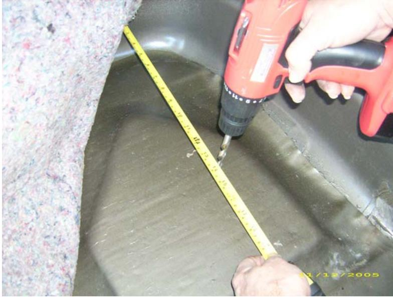
After drilling the starting hole at the 8" by 13-1/2" location, use a set of left and right cutting aviation snips or similar, and cut a spiral hole in the trunk floor approximately 4-3/4" to 5" diameter, exposing the pump mount and fuel connections.
