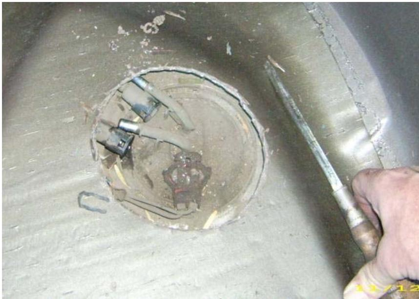
Remove the electrical connector and set aside.
