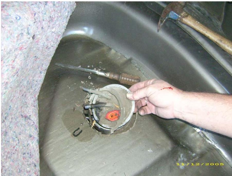
Carefully remove the pump & strainer assembly from the fuel tank. Retainer ring is shown to the left of the pump assembly
