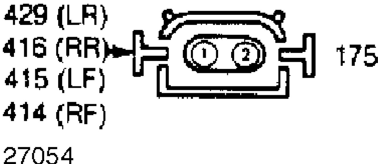
Fig. 5: Spring Solenoid Circuit Numbers
